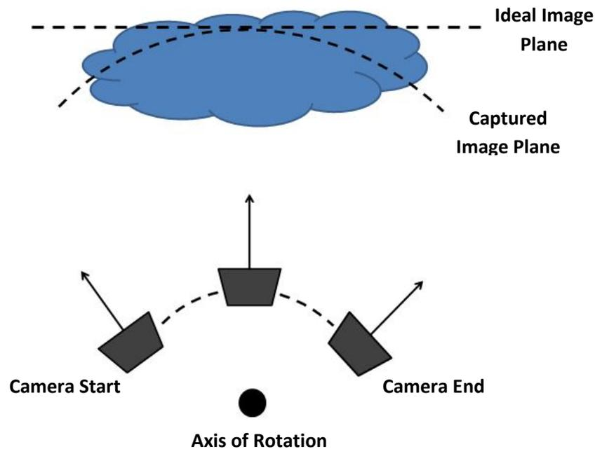
Figure 4: Schematic of Camera Orientation
