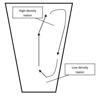
Figure 1: The flow pattern of the bubbles in the pint glass show how the bubbles rise in the center of the glass and begin to travel downward as they encounter the higher density region that causes the bubbles to sink under their own gravity. The density then decreases as the bubbles settle near the bottom of the glass, causing them to rise.
