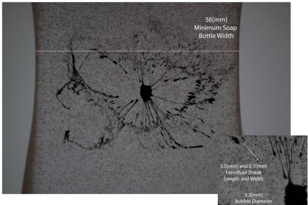
Figure 2: Top Left -Original image with measured reference scale Bottom Right- Magnified view with key extrapolated lengths
