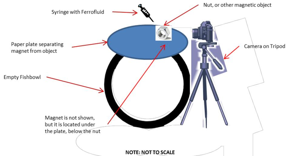
Figure 2 - Apparatus set-up
