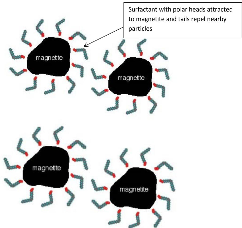
Figure 4 – Outcome of preparation of ferrofluid (adapted from [1])
