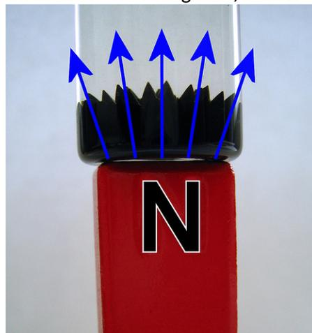
Figure 3 - Shows the north pole of a magnet repelling the ferrofluid (taken from [2])
