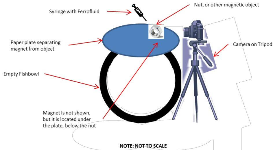
Figure 2 - Apparatus set-up
