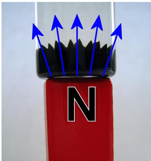
Figure 1 - Magnetic field lines shown by spikes in ferrofluid
