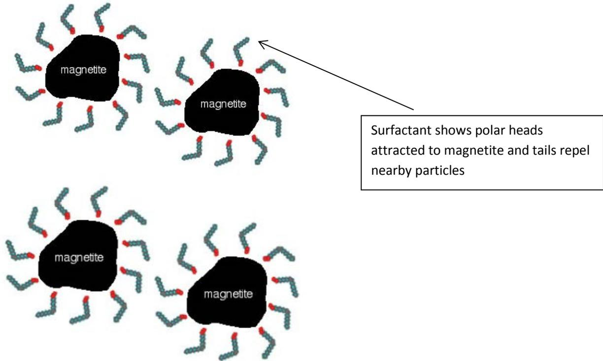
Figure 2 - Steric repulsion from interaction between surfactant and magnetite
