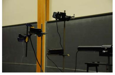
This image was taken in the dark with some lighting from adjacent rooms. The tank was filled with a mixture of cold tap water and pine-sol. The pinesol increases the visibility of the laser light in the water due to the size of the pinesol particles. The lighting in the image came solely from the laser light and ambient lighting from rooms around
