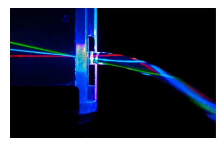
The purpose of this image was to show how light gets trapped in a laminar stream of water. The intent was to show how water essentially acts like a fiber optic cable with light. We actually got the idea from a youtube video that showed the same phenomenon. With the help of my team, Faith Batrack, Chris Franklyn, Jiffer Harriman, and David Gange as well as the physics department I was able to construct the setup to create my image.
