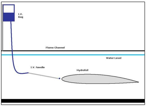
**Figure 1. Experimental Schematic**
