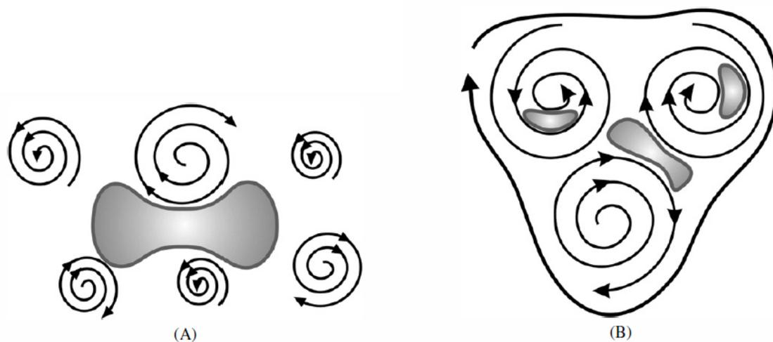
Figure 2: “Schematic presentation of the two regimes of emulsification in turbulent flow. (A) Turbulent inertial regime—the drops are larger than the smallest turbulent eddies and deform under the action of the fluctuations in the hydrodynamic pressure. (B) Turbulent viscous regime—the drops are smaller than the smallest turbulent eddies and, therefore, deform under the action of viscous stress inside and between the eddies.” [Vankova]
