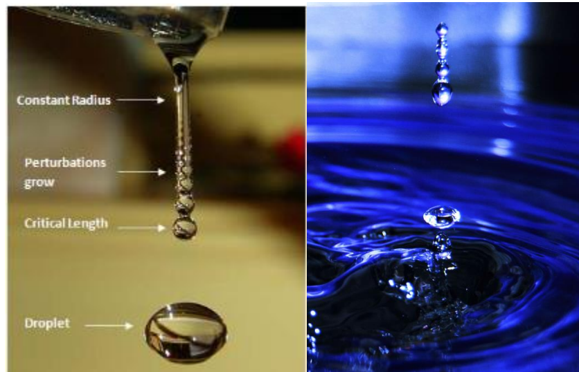
Figure 3: Comparison of images displaying Rayleigh-Plateau instability. Image from Breslouer, 2010 on left. Image from Kennedy, 2014 on right.
