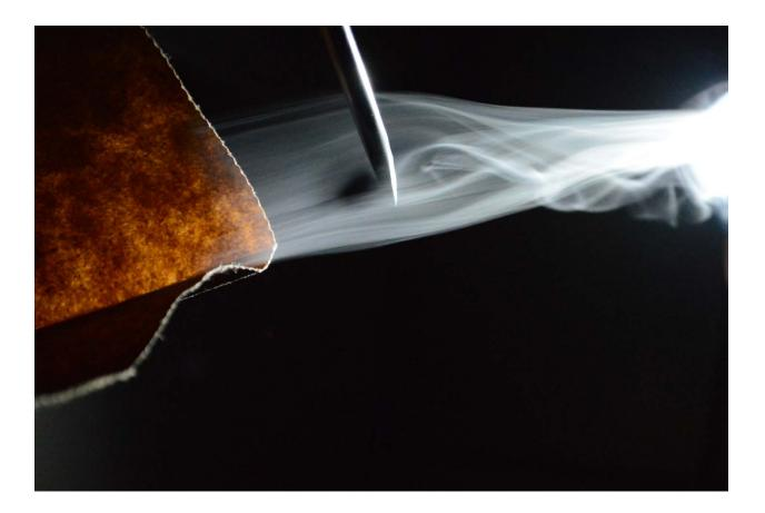
This photograph was taken for the first assignment, Get Wet, in the University of Colorado's Flow Visualization course. The intent of this individual assignment was to get the student's feet wet in photography and flow visualization. For this image I attempted to capture the transition from laminar to turbulent flow.
