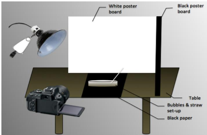
Figure 2. Demonstration of imaging set-up.
