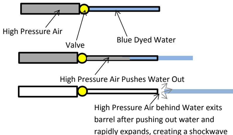
I believe this is what caused the glass to shatter, as the cannon made a loud explosion noise once the water was expelled completely, and the glass shattered directly after that event.
