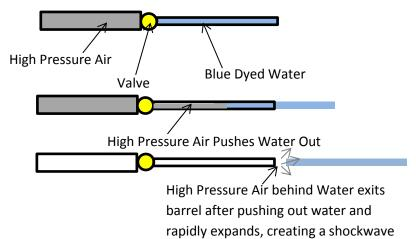
The air cannon shockwave was formed as shown below:
