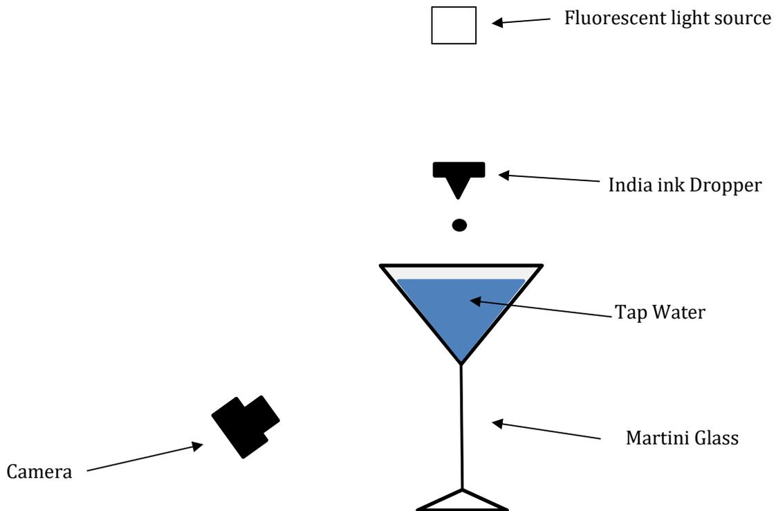
Figure 1: Flow Setup Diagram
