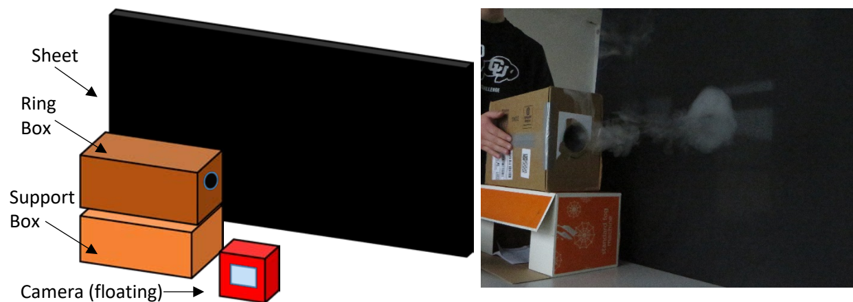
Figure 1: Animated experimental setup (Left), Realistic experimental setup (right)
