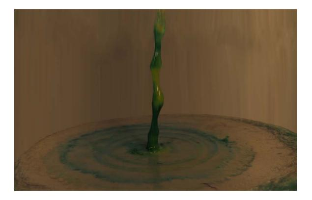
The image shown above was taken for the first flow visualization team project at the University of Colorado at Boulder. It illustrates the motion of India ink falling through water and impacting a metal plate set horizontally on the ground. The primary properties exhibited in this image include hydraulic jumps, cohesion, and surface tension.
