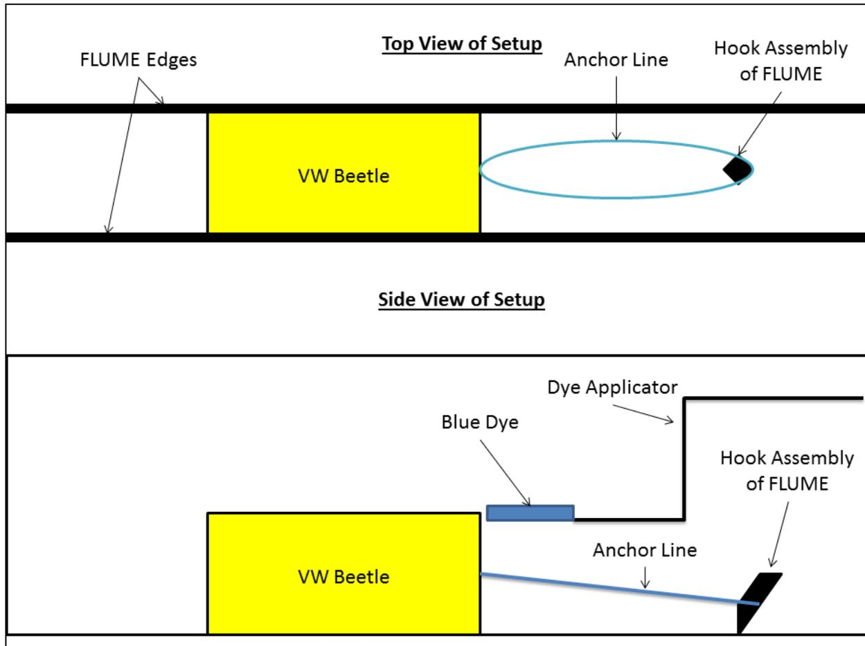
Figure 3-Top and Side View Schematic of FLUME setup for Team Photo #1
