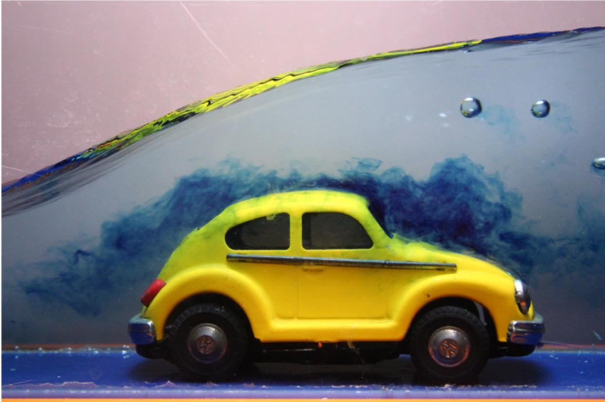
Figure 6-Original Unedited Photo detailing Fluid Flows Over a VW Beetle in a FLUME
