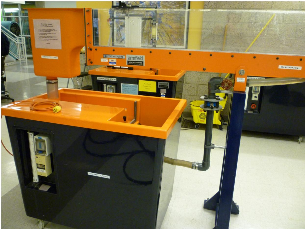
Figure 2-Basic overview of the FLUME used for the purposes of determining fluid dynamics
