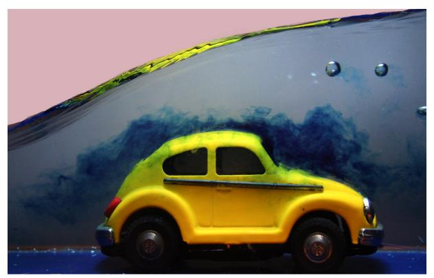
Figure 1-Application of Blue Dye in a FLUME for a VW Die Cast Model
