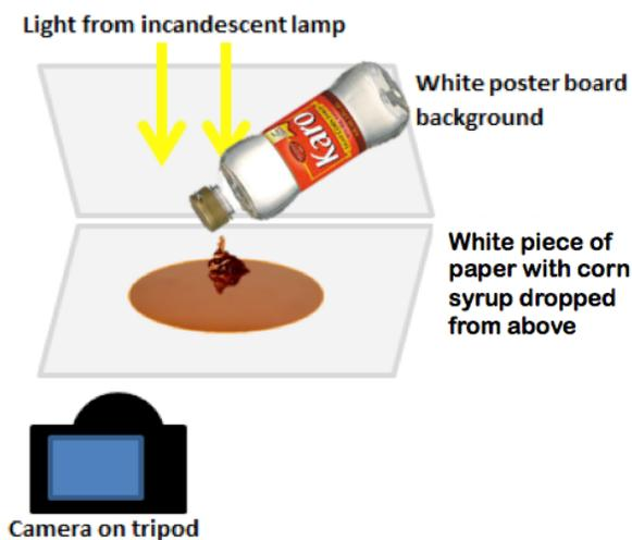
below. The flow itself was created using Karo Corn Syrup that was dyed purple, poured in a cup, and placed in the freezer for about 10 minutes to make it cooler and therefore, more viscous. Corn syrup was chosen because of its high viscosity and ability to fall in a steady stream with varying
