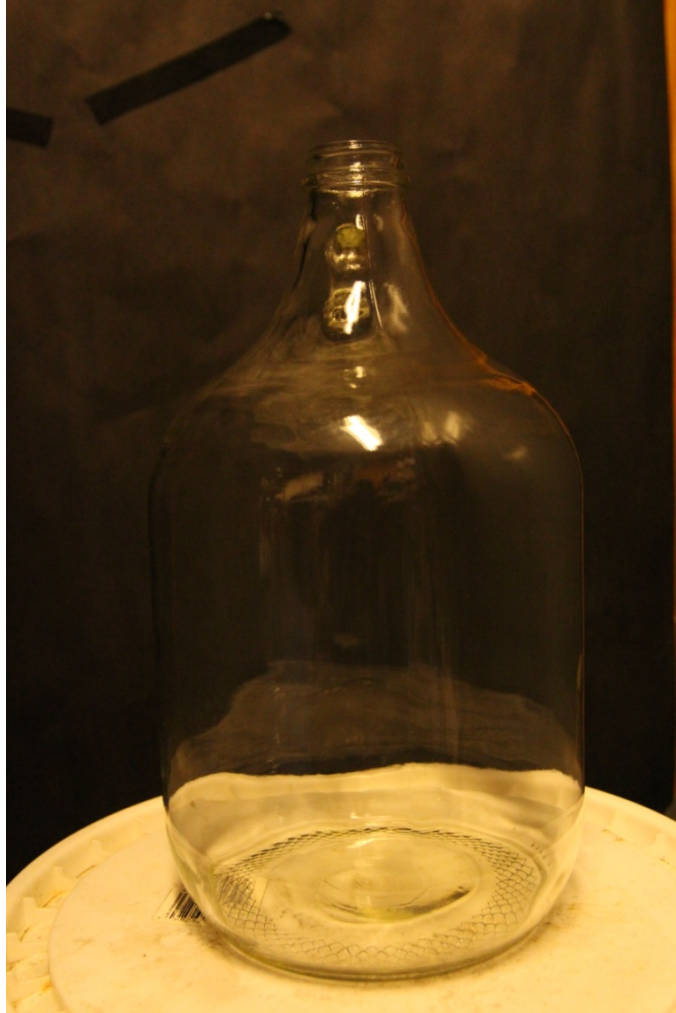
Figure 1 Jar used for flame propagation experiment
