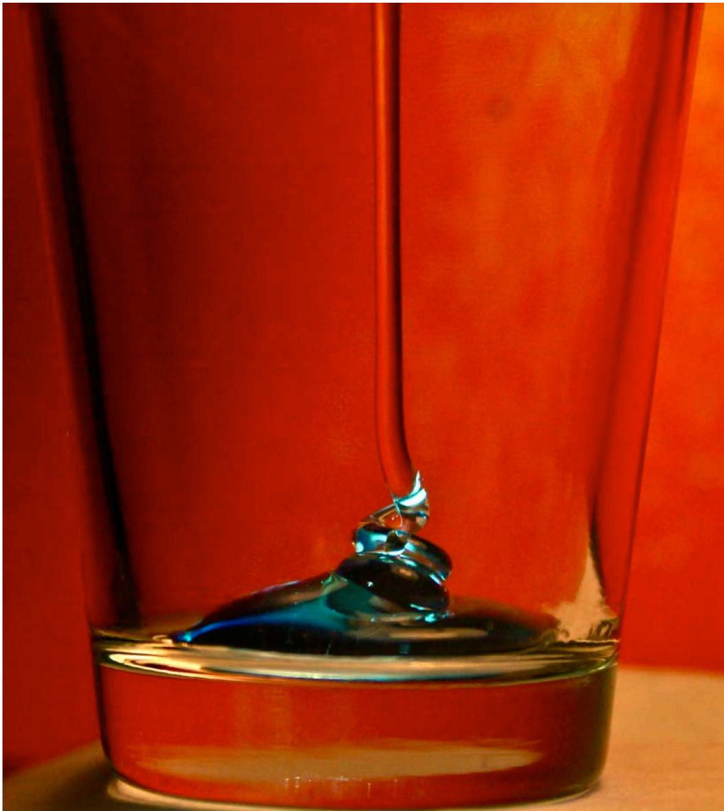
The purpose of this image was to continue team-centered exploration into the world of flow visualization. The intent of this image was to capture a fluid phenomenon in a visually appealing way, whilst exploring personally unknown territory. I was unsure of which regime of the rope-coiling effect I wanted to capture (inertial or gravitational) so I took many pictures to find one that I liked.
