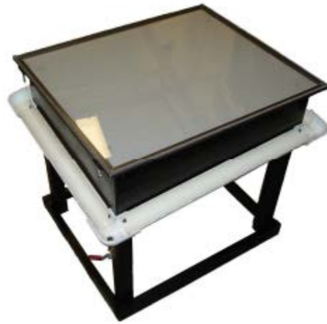
Figure 1: The Hele-Shaw cell used 1
