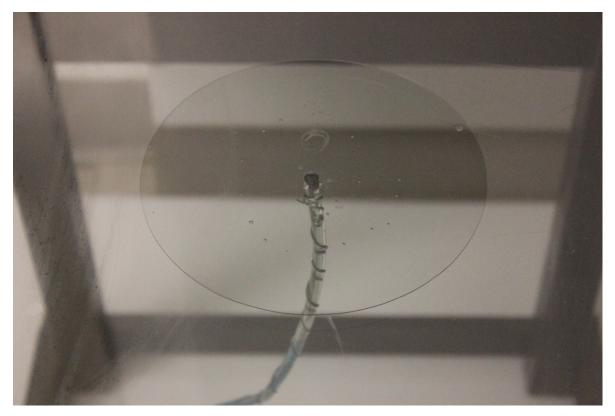
Fig 2: Initial condition in a Hele Shaw cell with corn syrup.
