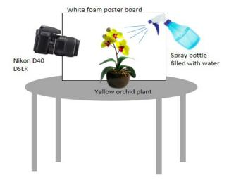
Figure 1. Schematic of flow imaging set-up.
