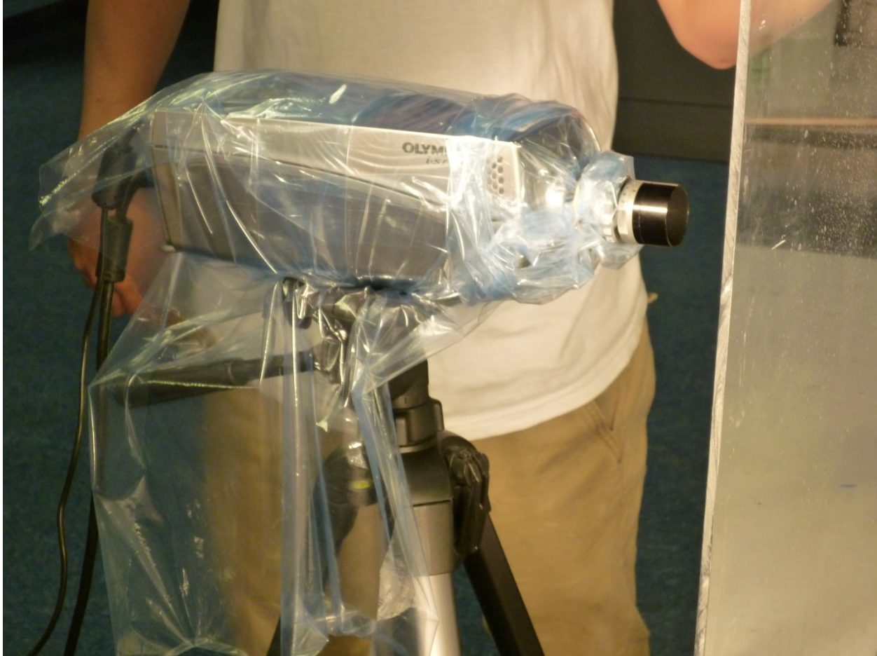
Figure 2-Olympus High Speed Camera used for the experiment. Camera was protected with plastic wrap.
