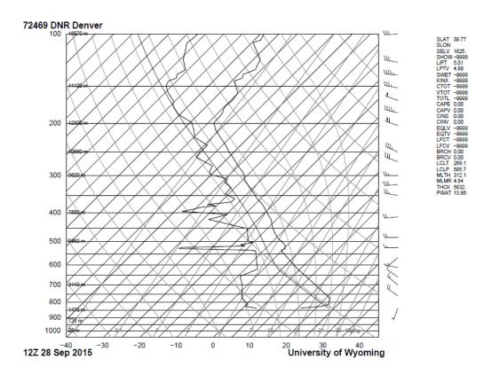
Figure 1: Skew-T Diagram for September 28<sup>th</sup>, 2015 12Z from Denver International Airport
