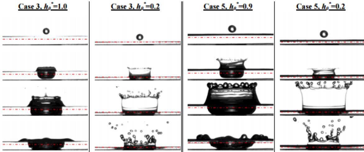
Figure 1 Crowning effect of Weber Number from Hillen's Droplet Impact Time Histories
