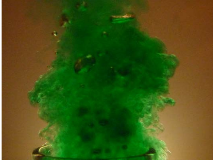
Figure 3: Dyed vegetable oil dropped in water. This image was captured without the camera flash but used a camping light behind the tank. Also, no toilet paper was in the tank.
