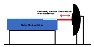
*Figure 2: The speaker on the right, connected to the open container.*
