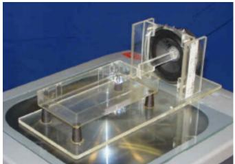
Figure 1: The Capillary Wave Generator. Image courtesy of Jean Hertzberg.
