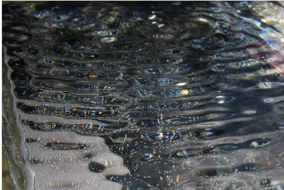
Final Group Project 1 Image: Faraday waves in water excited at a frequency of 8 Hz.
