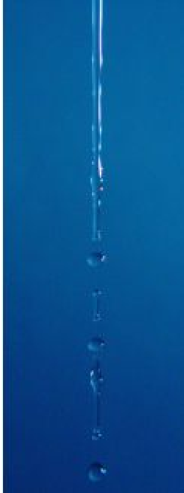
Fig. 2 The Rayleigh instability effect as seen in a water thread falling under the influence of gravity. The initial jet diameter is approximately 3 mm [2].
