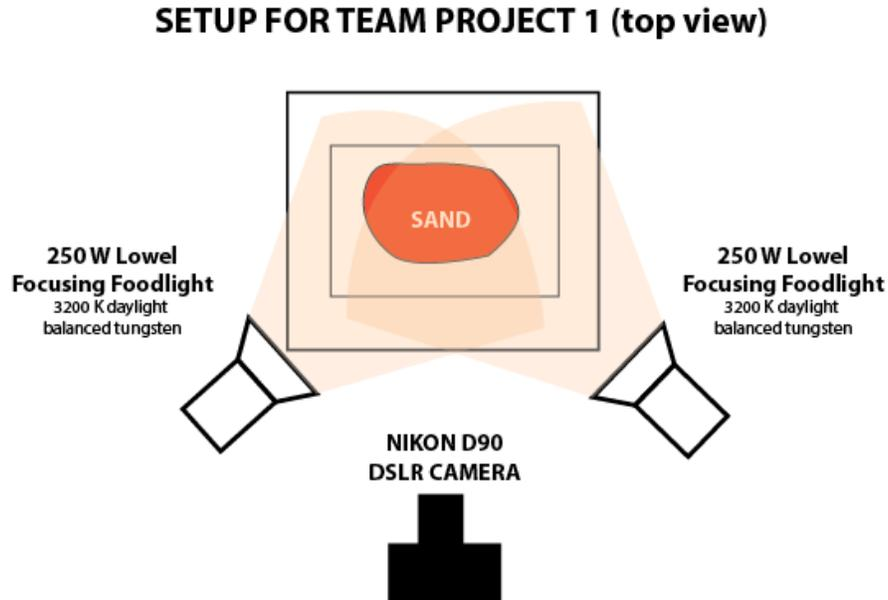
Figure 3: Diagram of setup.
