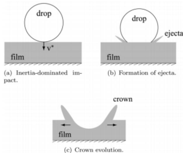
Figure 2: Evolution of a crown splash.
