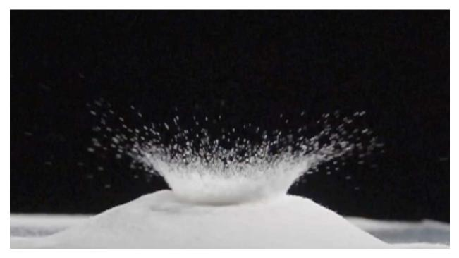
Figure 1: Single frame from video shows the granular crown splash.
