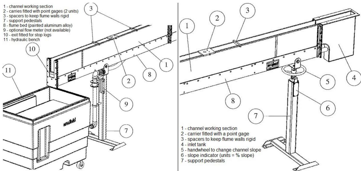
Figure 1: Armfield Open Channel Flume
