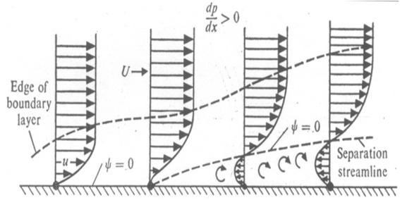
Figure 4: Flow Separation [7]
