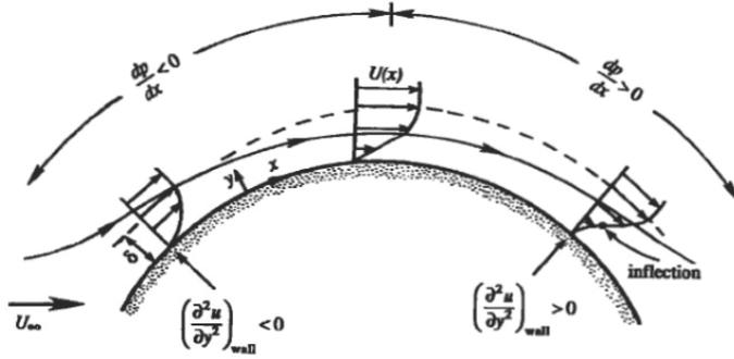
Figure 3: Flow Past a Cylinder [7]
