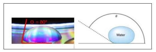
Figure 4: Contact Angle of Water Drop on CD Surface<sup>3</sup>
