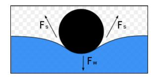
Figure 3: Free Body Diagram of Water Bead on CD Surface<sup>4</sup>
