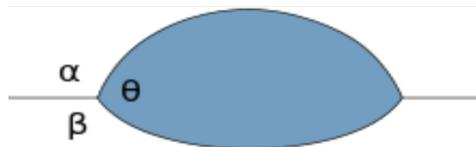
Figure 4: Coexistence of three fluid phases in mutual contact:  $\alpha$ ,  $\beta$ , and  $\theta$  represent both the labels of the phases
