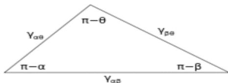
Figure 5: Neumann's triangle relating the surface energies and contact angles of three fluid phases coexisting in static equilibrium, as depicted in Figure 4
