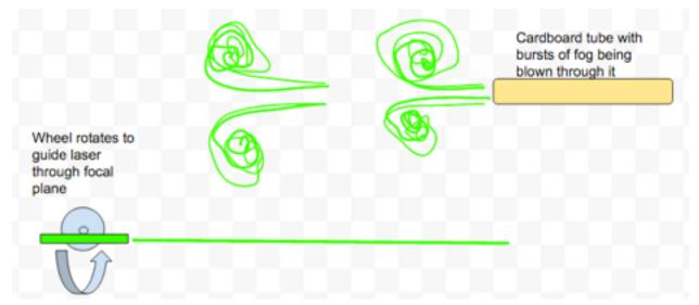
Figure 1: Depiction of experimental set up with camera 3.5 ft out of the page.
