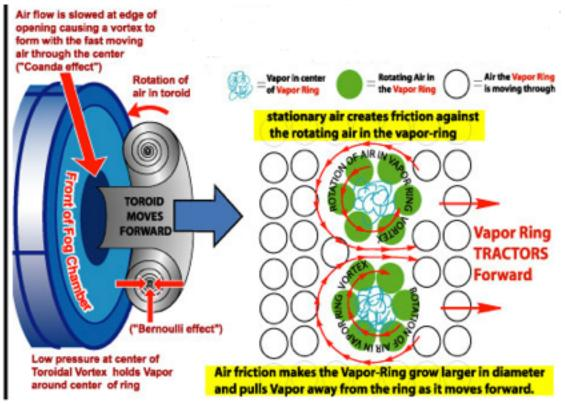
Figure 2: Depiction of spiraling motion and explanation of vortex formation.<sup>1</sup>
