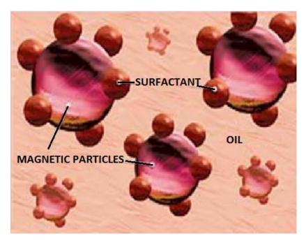
Figure 4: Magnetic particles, with surfactant molecules attached, suspended in a oil fluid to form a ferrofluid. The surfactant prevents clumping of the magnetic particles. (Drawing from Ferrotec Corporation [USA])<sup>7</sup>.
