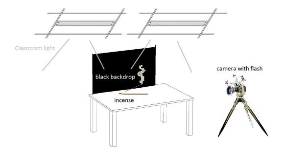
Below is the set up we should have had to prevent the light washing out details. External flashes should have been on the both sides of the incense, with no flash coming from the front.
