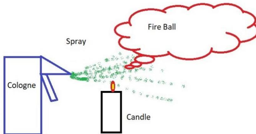
Figure 1: The set up to capture the fireball image.
