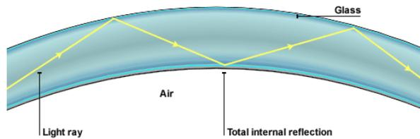
Figure 5: Sketch of total internal reflection from [3]
