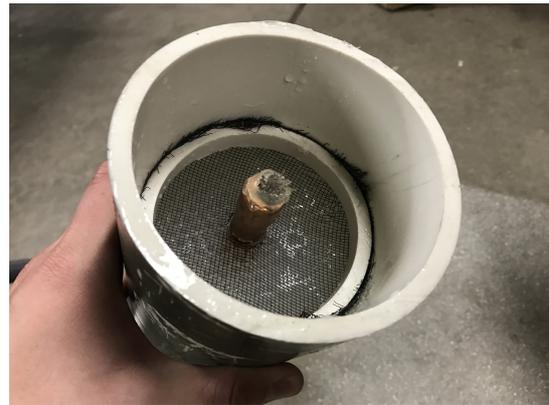
Figure 3: Inside view of straw array and copper tube containing fiber optic strands
