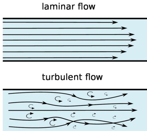
Figure 1: Sketch of Laminar vs. Turbulent flow from [1].
