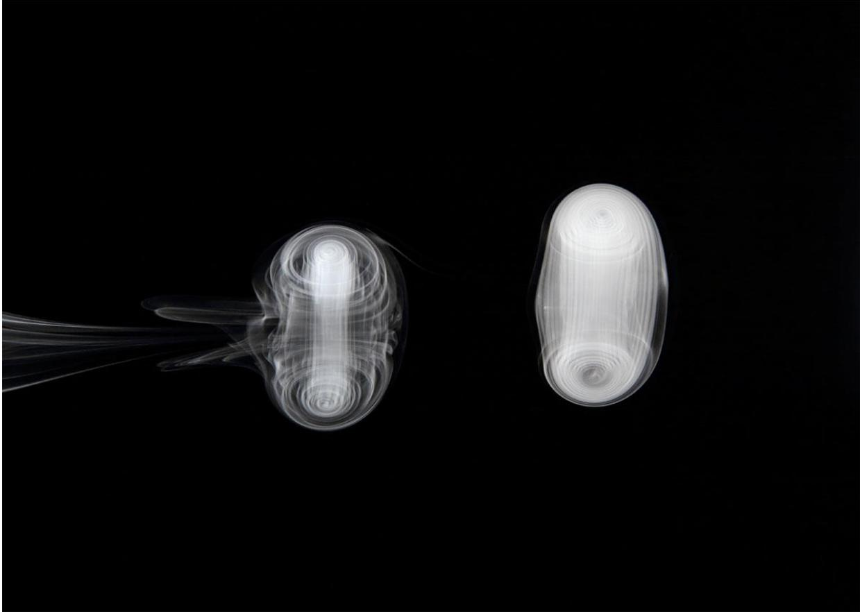
Figure 3: Photo of two circular vortex rings propagating left to right seeded with smoke
