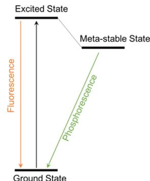
Figure 1: Light Emission from Excited State
