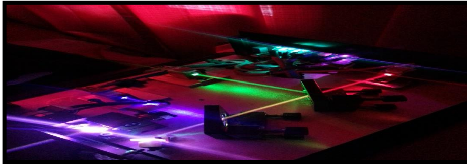
Figure 2 – The combination of the three laser diode beam emissions
