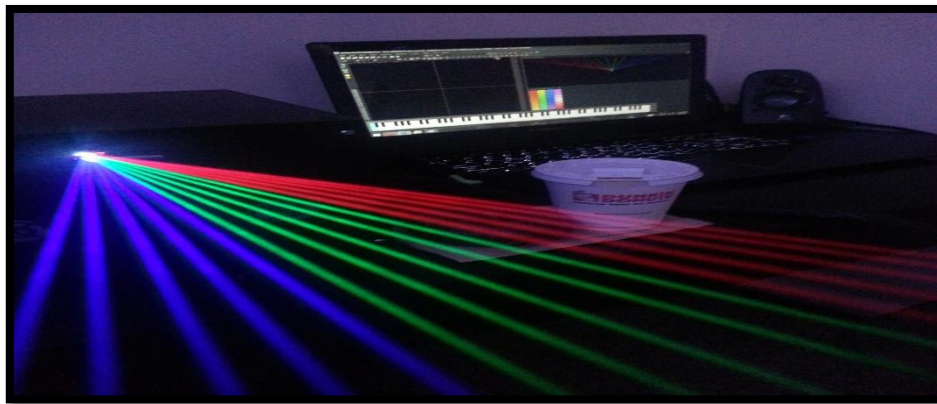
Figure 3 – An output at the aperture shows the R, G, and B beams combined at the scanner pair
