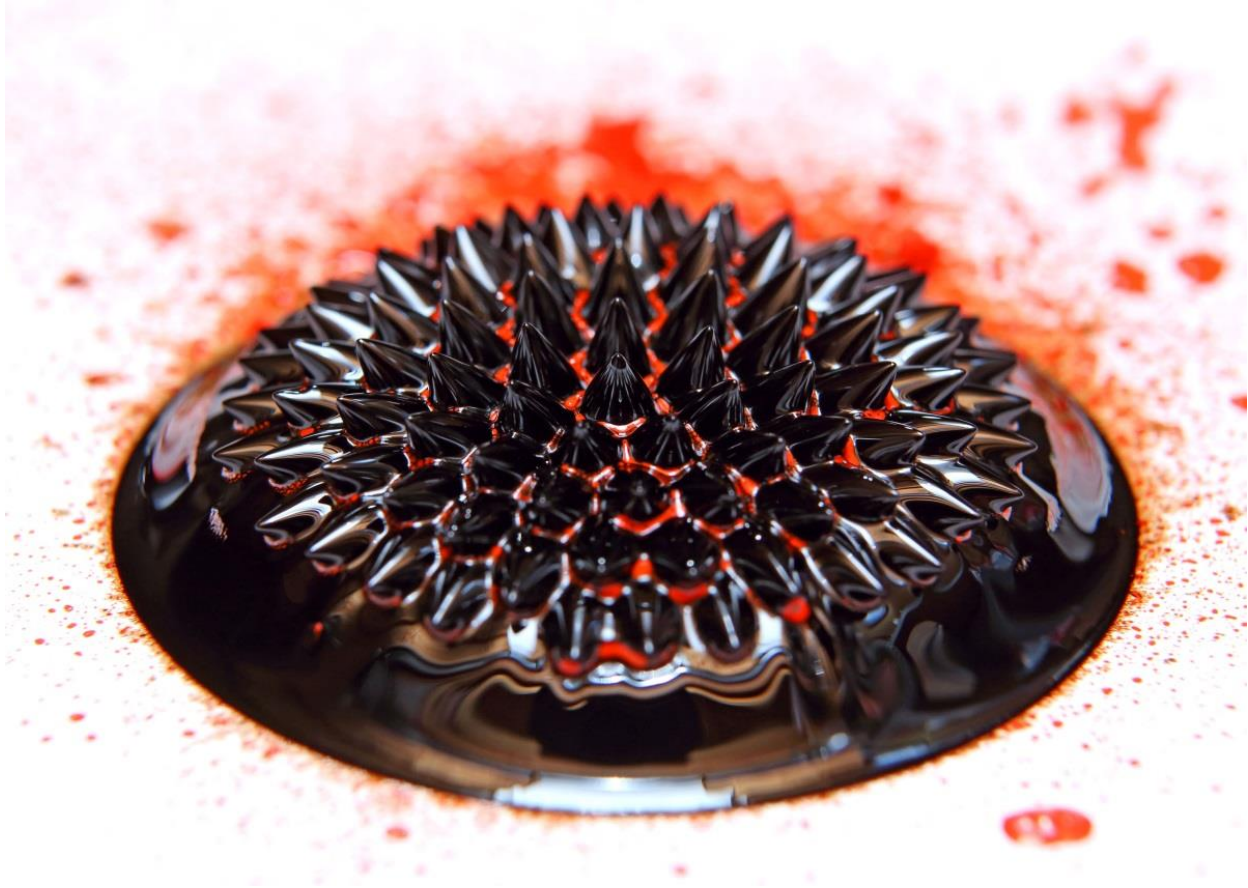
Figure 2: Ferrofluid under the influence of a magnetic field and covered with droplets of India ink
