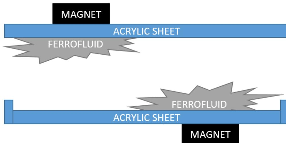
*Figure 1: Apparatus setup showing the relative placement of the magnets and ferrofluid.*
