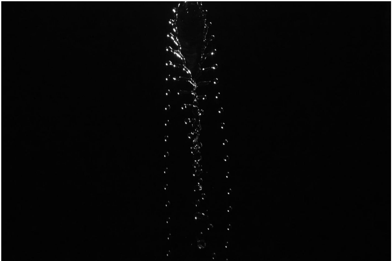
Figure 1: Fishbone Structure Formed by Two Colliding Jets
