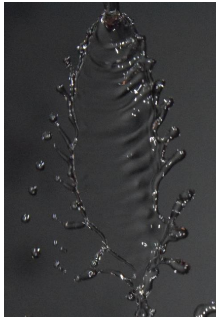
Figure 7: A clear representation of an oscillation in the sheet of fluid
