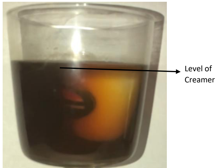
Figure 2: Rayleigh-Taylor instability in cold creamer and hot coffee
