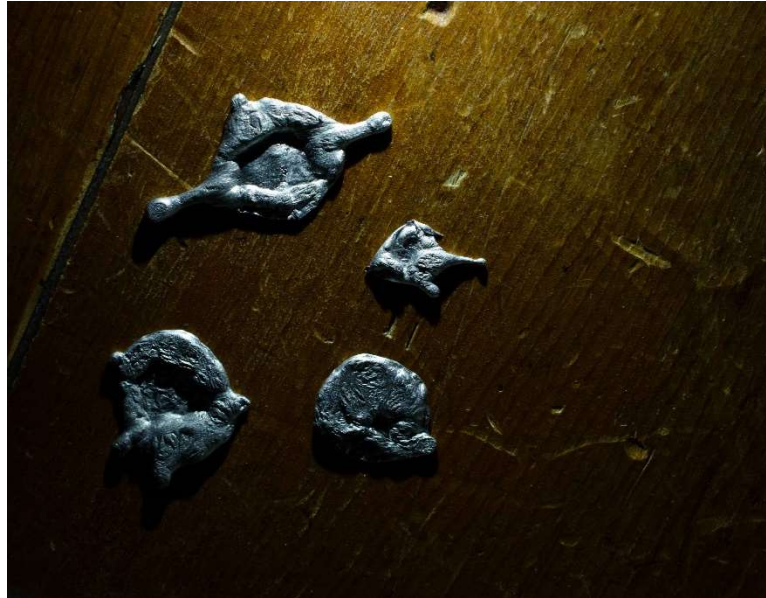
Figure 1: All the different drops collected during TIG welding
