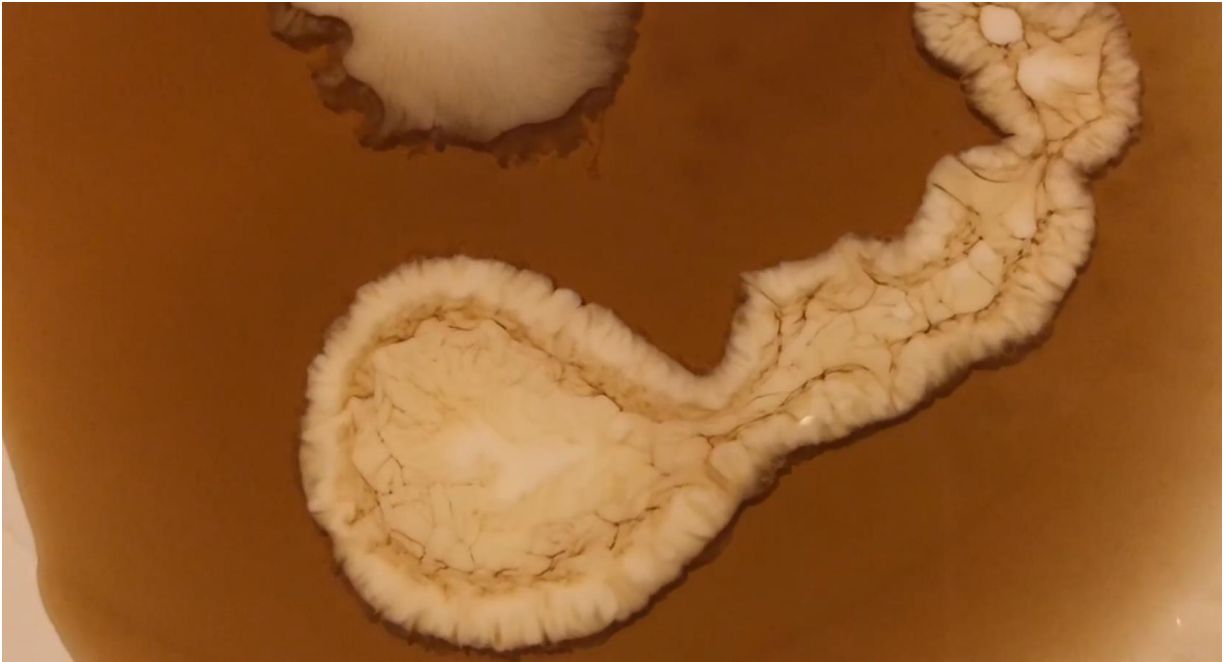
Figure 5: Solutal convection cells in second half of the video
