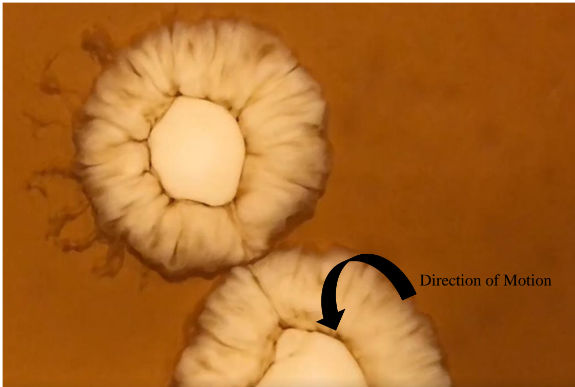
Figure 4: Convection cells formed by solutal convection
